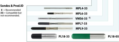
Shock absorbers are special accessories to Vesala's NanoSonde, MicroSonde and MiniSonde, intended for duct tracing and calibration together with a blowing machine. They considerably decrease risk of sonde damage during jetting by absorbing the excessive energy when the sonde hits an object. Hence it is recommended to use shock absorbers when possible.
