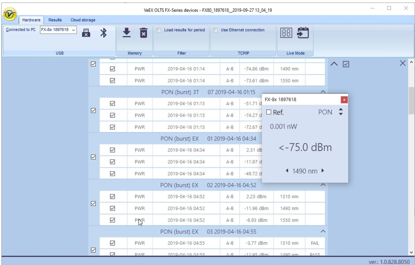
3. Use the box to control the measurement just like from the power meter. For more information about the meter's operation, see the corresponding User Manual at [www.veexinc.com](http://www.veexinc.com).
