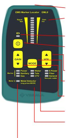
**Antenna connector:** To connect EA3 search coil antenna with AK1 cord and adapter.
