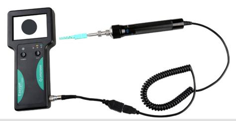
Easyget 2 is a portable type of fiber endface inspector developed by Dimension Technology. By magnifying 200~400 time of the objects, you can identity defects and scratches on the endface of connectors. It is your the best choice for endface inspection. Easyget comes along with portable 3.5 inch high resolution LCD monitor, it can work over 8 hours after recharge. There are also all kinds of tips which make Easyget to meet different requirements on inspecting.
