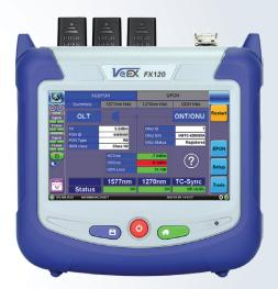
The FX120 is an all-in-one advanced PON analyzer with an Ethernet interface and an SFP+ cage to support Layer 4+ testing. Monitor activation process by displaying downstream/upstream power levels as well as OLT/ONT IDs and status and TC-Sync. Certify QoE using Speed Test and V-PERF to check internet connectivity and speed up to 10 Gbps. Optional Fault Locator feature allows technicians to check drop cables.
