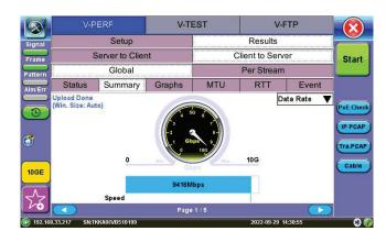
V-PERF is a hardware-based benchmarking test for network performance at different TCP window sizes, to verify stateful TCP/UDP throughput at full line rate, understand KPIs that may be causing network congestion and speed degradation, optimize window sizes, and assure the link meets the required quality of service (QoS)
