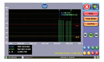
Toggle Channel units between wavelength or frequency. An active channel threshold is available to allow users to control which channels to display in the table.
