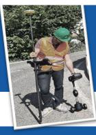
The MRT-700 is also used by topography companies where **extremely high precision** is required by connecting the device to an **external GPS**.
