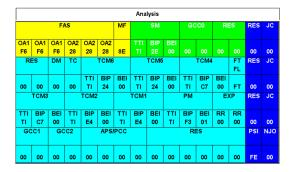
Overhead byte control allows the manipulation and easy encoding of transmitted overhead bytes in both terminated and payload through modes to stress the network responses to various conditions.
