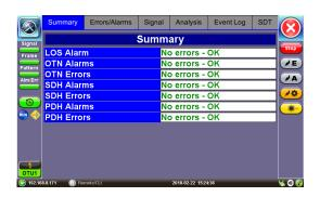
Alarms and Errors overview with history indicators provide direct (touch) access to counters and statistics and complement the soft LEDs with a layered representation of all defects and anomalies.
