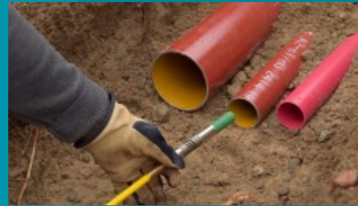
The 512 Hz sondes can be used in either plastic or metal pipes. The 33 kHz sonde is designed for plastic pipes.
