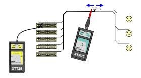
A certain pair is easy to find e.g. at a cable joint with the XT25. This is useful when reserved pairs in a cable have to be traced and taken into use.
