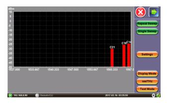
The Repeat Sweep allows the user to drill down specifically into a single channel view to monitor continuous channel performance including signal level, laser drift and OSNR. The user can move the cursor to go back in time to reverify signal anomalies that recently occurred.
