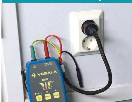
...or use the special Schuko cord to trace wall socket wirings...
